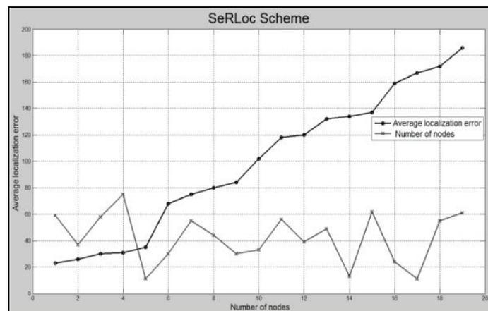
Figure 3. Number of nodes Vs Average localization error for SeRLoc scheme.
