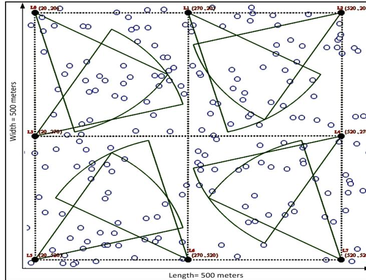
Figure 1. The Grid based network model with eight locator nodes
