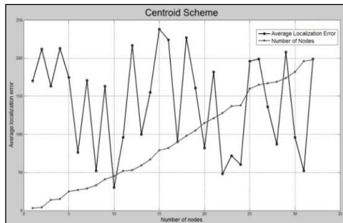
Figure 2. Number of nodes Vs Average localization error for Centroid scheme
