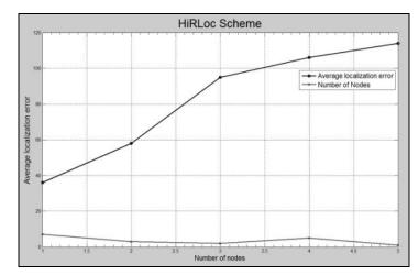
Figure 4.Number of nodes Vs Average localization error for HiRLoc scheme.
