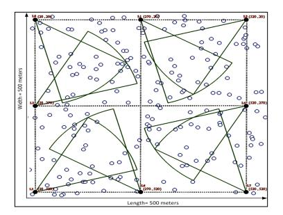
Figure 1.The Grid based network model with eight locator nodes
