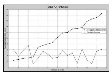
Figure 3.Number of nodes Vs Average localization error for SeRLoc scheme.
