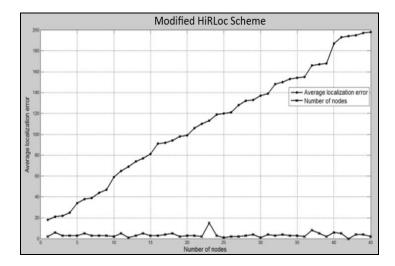
Figure 5.Number of nodes Vs Average localization error for modified HiRLoc scheme.
