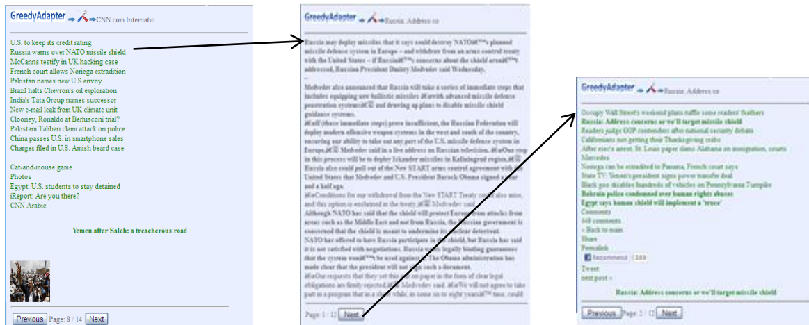
Figure 10. (a) The adapted CNN page by GreedyAdapter on handheld before navigating “Russia warns over NATO missile shield”, (b) the first subpage of adapted version of the navigated page, (c) the second subpage of the adapted page.
